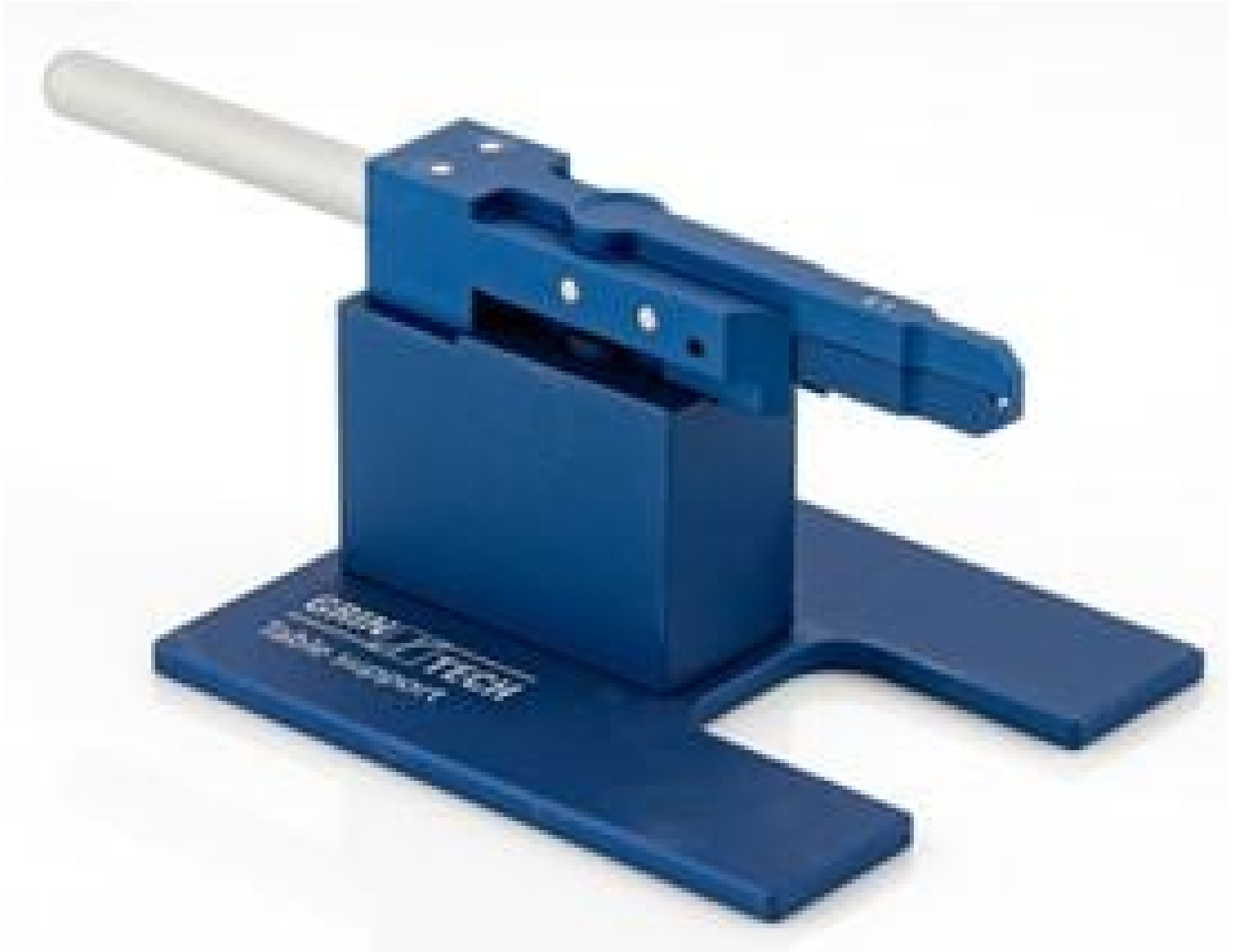
GRIN Lens Gripper w/Table Mount 27mm Height
