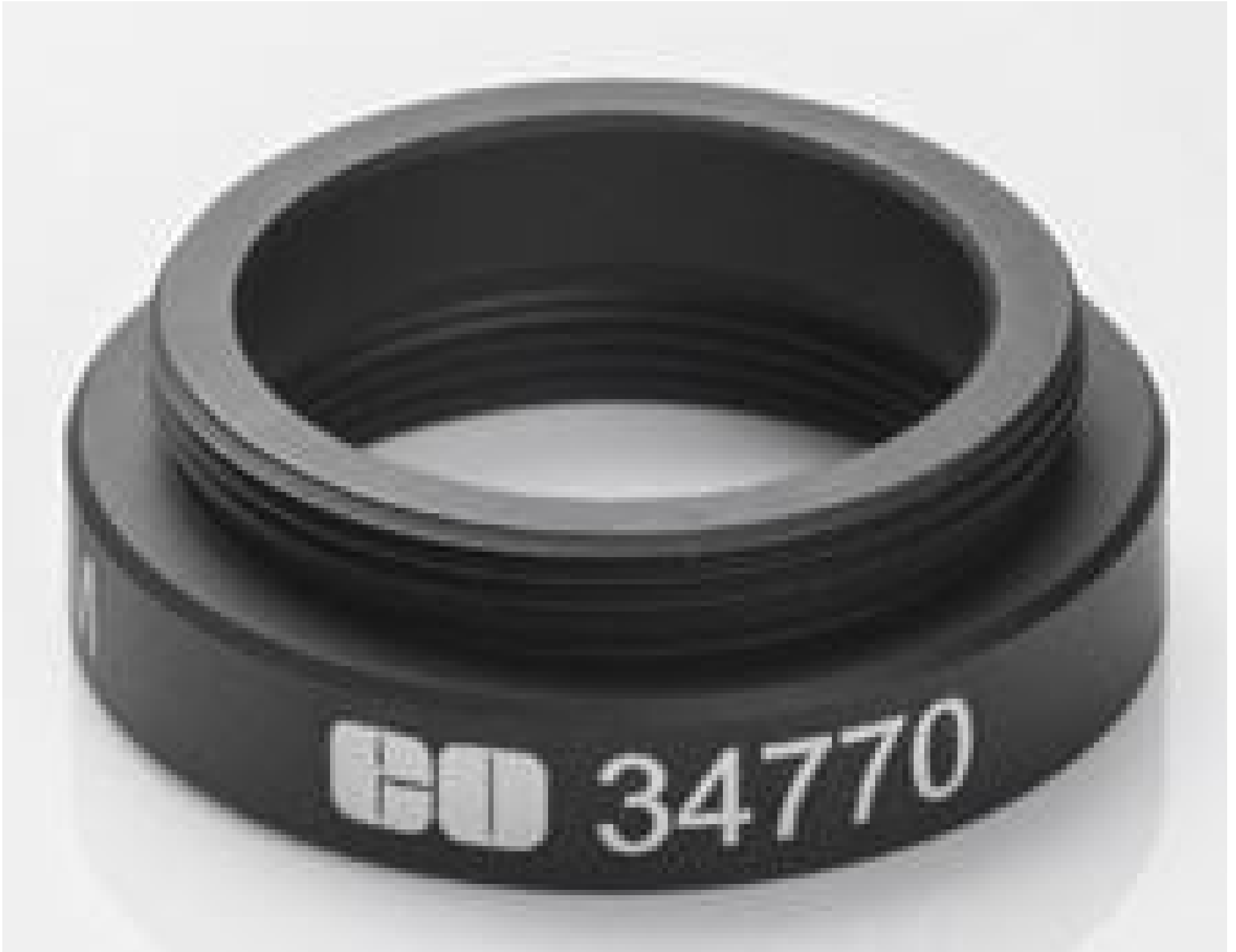
Female M22 x 0.75 to Male C-Mount Adapter, #34-770
