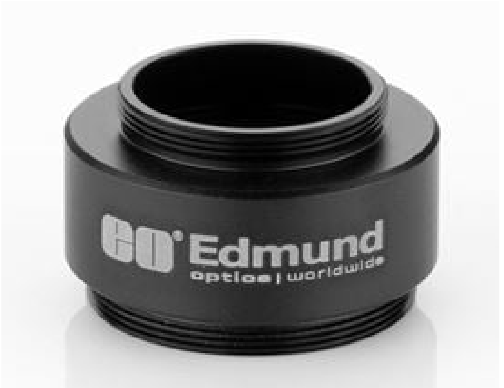
Female C-Mount to Male M32 x 0.75 Adapter
