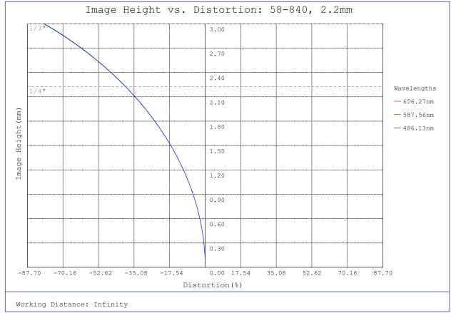
#58-840, f/2.0, Visible, 2.2mm HEO Series M12 Lens, Distortion Plot
