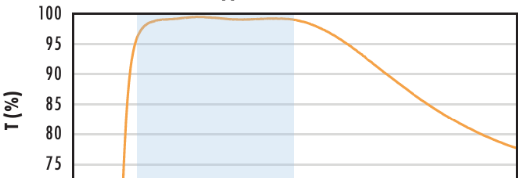
N-BK7 with VIS-EXT Coating Typical Transmission
