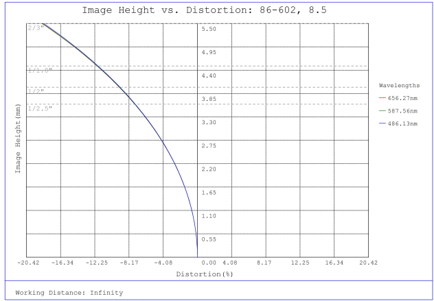
#86-602, 8.5mm, f/4 Ci Series Fixed Focal Length Lens, Distortion Plot
