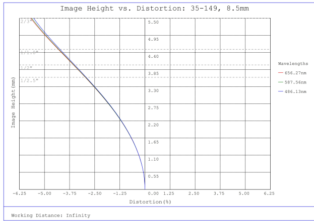
#35-149, 8.5mm, f/2.8, 75mm-∞ Primary WD, HRr Series Fixed Focal Length Lens, Distortion Plot
