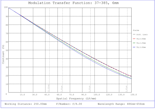
#37-385, 6mm FL f/8.0, Rugged Blue Series M12 Lens, Modulated Transfer Function (MTF) Plot, 250mm Working Distance, f8
