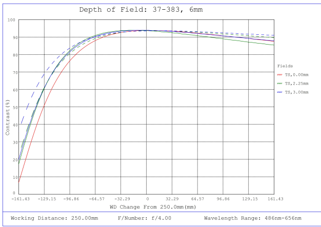
#37-383, 6mm FL f/4.0, Rugged Blue Series M12 Lens, Depth of Field Plot, 250mm Working Distance, f4
