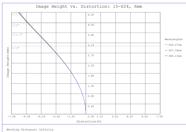
#15-624, 6mm, f/8.0 Cw Series Fixed Focal Length Lens, Distortion Plot
