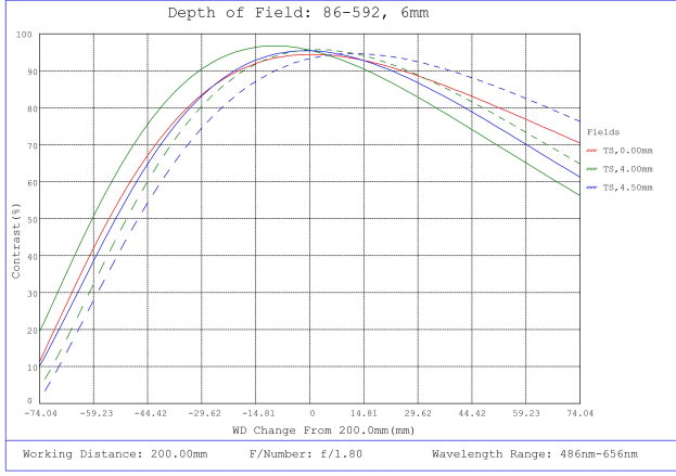
#86-592, 6mm, f/1.8 Ci Series Fixed Focal Length Lens, Depth of Field Plot, 200mm Working Distance, f1.8
