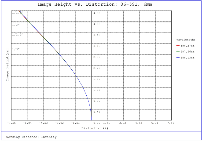
#86-591, 6mm, f/1.4 Ci Series Fixed Focal Length Lens, Distortion Plot
