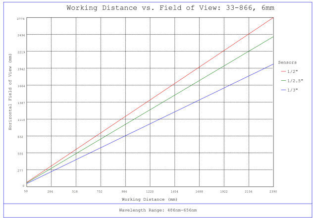
#33-866, 6mm, f/8 UCi Series Fixed Focal Length Lens, Working Distance versus Field of View Plot
