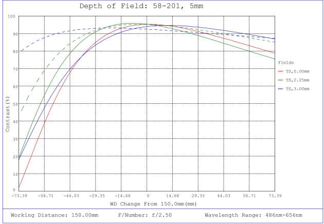
#58-201, 5mm FL f/2.5, Blue Series M12 Lens, Depth of Field Plot, 150mm Working Distance, f2.5
