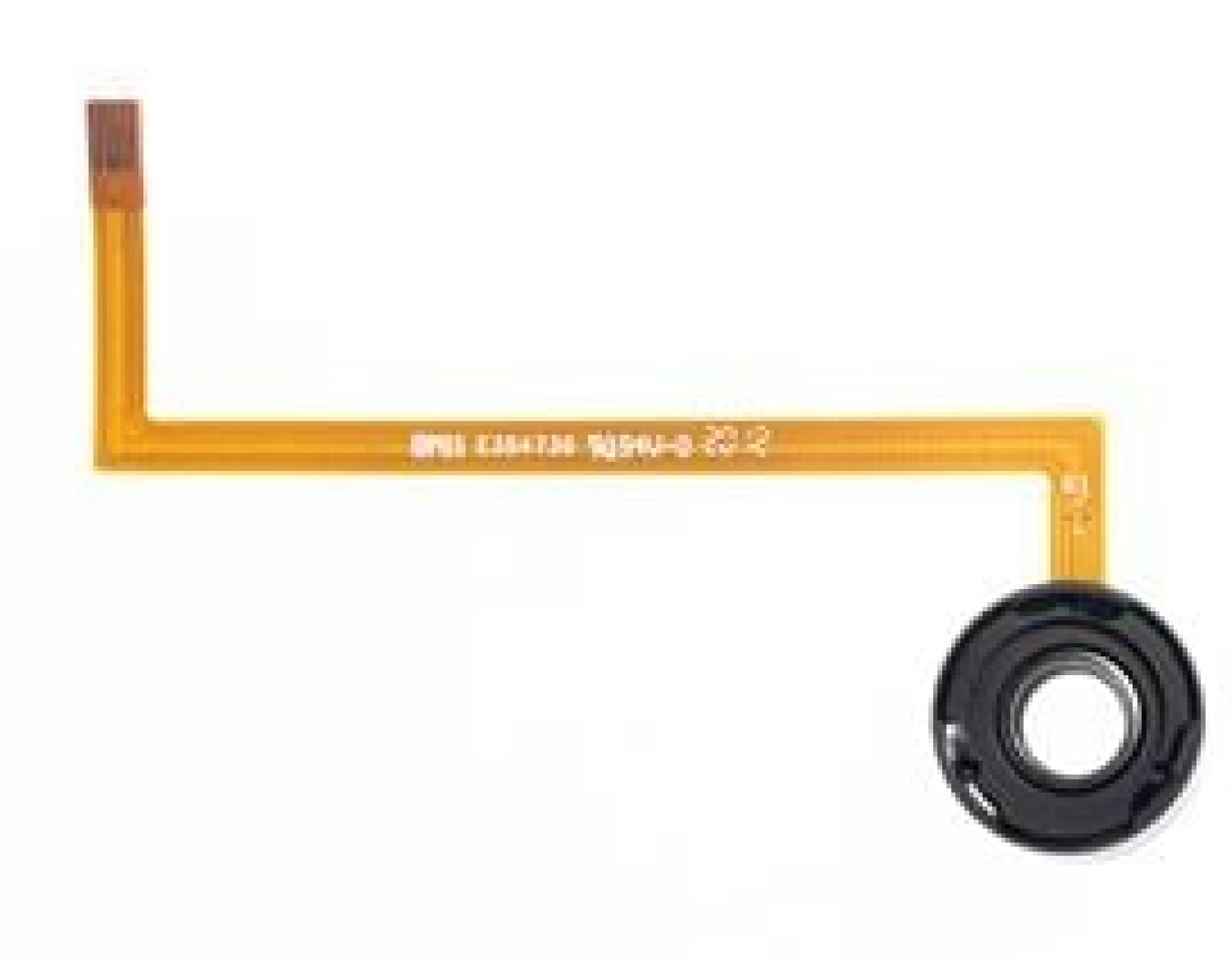
5.8mm CA, NIR Coated, A-58N1-P20 Corning® Varioptic® Variable Focus Liquid Lens, Packaged A-Series - 6 pins FPC with Thermistor
