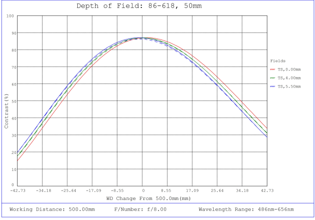
#86-618, 50mm, f/8.0 Ci Series Fixed Focal Length Lens, Depth of Field Plot, 500mm Working Distance, f8
