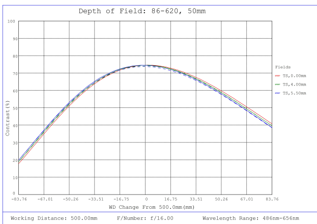
#86-620, 50mm, f/16.0 Ci Series Fixed Focal Length Lens, Depth of Field Plot, 500mm Working Distance, f16
