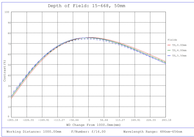
#15-668, 50mm, f/16 Sealed Cw Series Fixed Focal Length Lens, Depth of Field Plot, 1000mm Working Distance, f16
