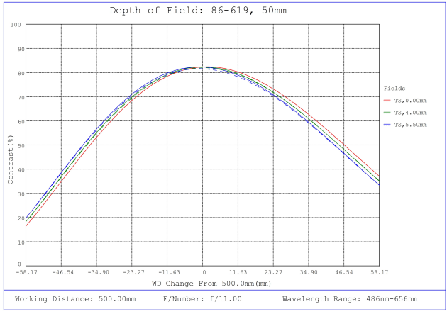
#86-619, 50mm, f/11.0 Ci Series Fixed Focal Length Lens, Depth of Field Plot, 500mm Working Distance, f11
