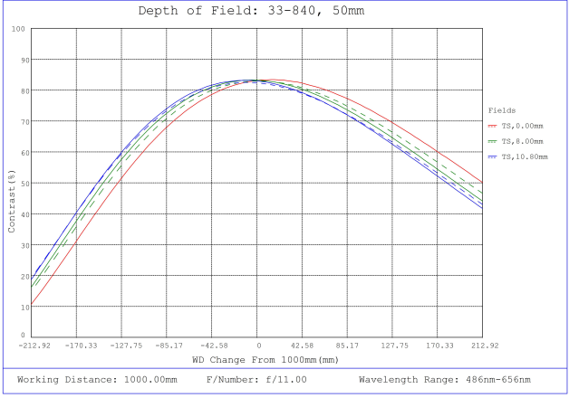
#33-840, 50mm f/11, HPi Series Fixed Focal Length Lens, Depth of Field Plot, 1000mm Working Distance, f11
