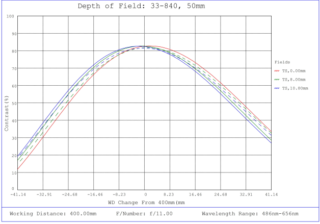
#33-840, 50mm f/11, HPi Series Fixed Focal Length Lens, Depth of Field Plot, 400mm Working Distance, f11
