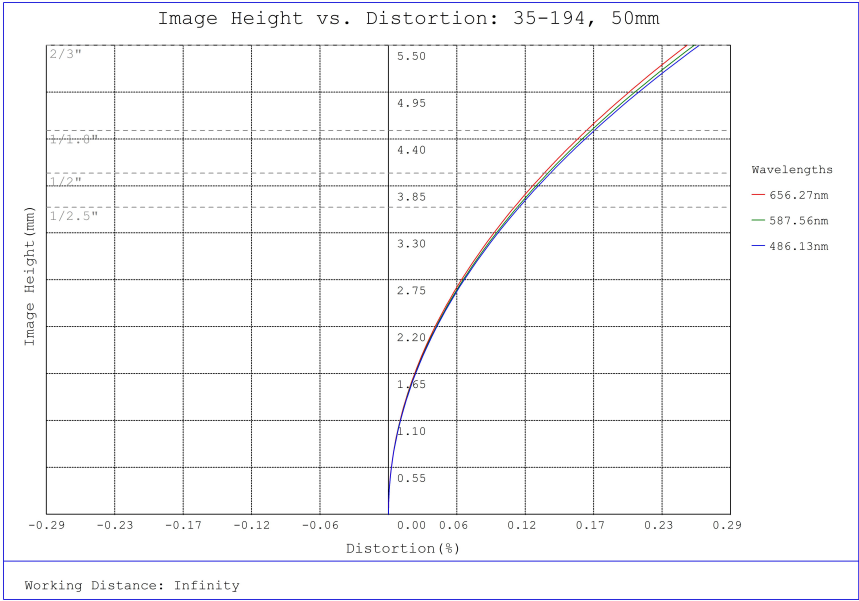
#35-194, 50mm, f/8.0 Cr Series Fixed Focal Length Lens, Distortion Plot
