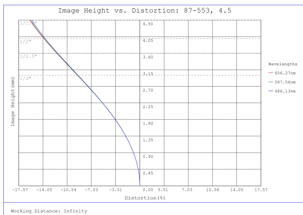
#87-553, 4.5mm, f/4 Ci Series Fixed Focal Length Lens, Distortion Plot
