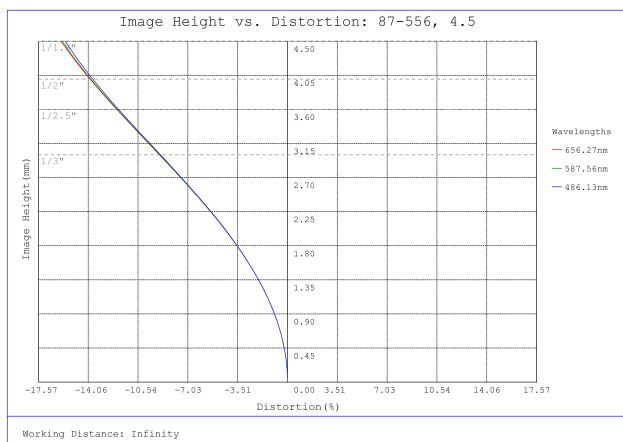
#87-556, 4.5mm, f/11 Ci Series Fixed Focal Length Lens, Distortion Plot
