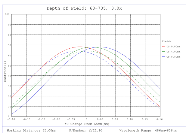
#63-735, 3X, 65mm WD CompactTL™ Telecentric Lens, Modulated Transfer Function (MTF) Plot, 65mm Working Distance, f21.9
