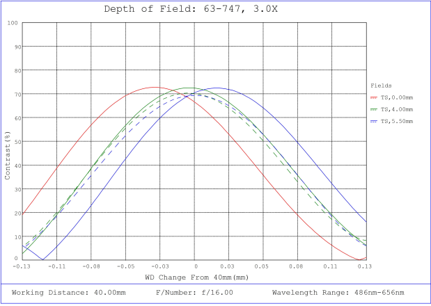
#63-747, 3X, 40mm WD CompactTL™ Telecentric Lens , Depth of Field Plot, 40mm Working Distance, f16
