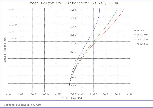
#63-747, 3X, 40mm WD CompactTL™ Telecentric Lens , Distortion Plot
