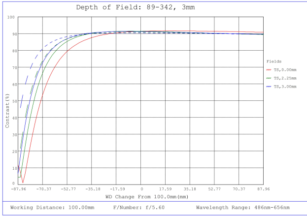
#89-342, 3mm FL f/5.6, Blue Series M12 Lens, Depth of Field Plot, 100mm Working Distance, f5.6
