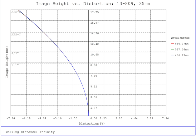
#13-809, 35mm TFL-II Mount LH Series Fixed Focal Length Lens, Distortion Plot
