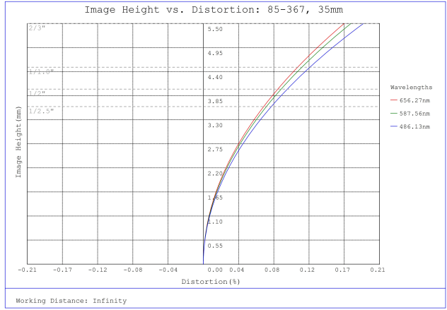
#85-367, 35mm, f/8 Ci Series Fixed Focal Length Lens, Distortion Plot
