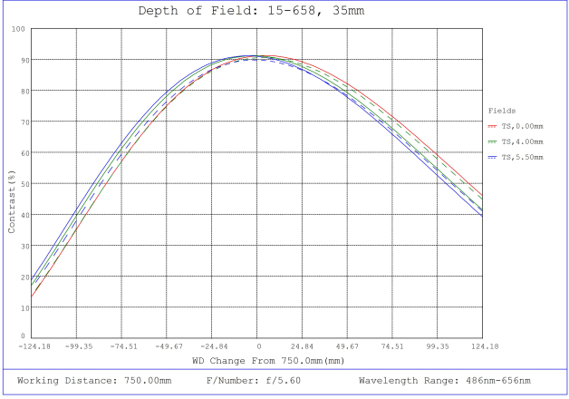
#15-658, 35mm, f/5.6 Cw Series Fixed Focal Length Lens, Depth of Field Plot, 750mm Working Distance, f5.6
