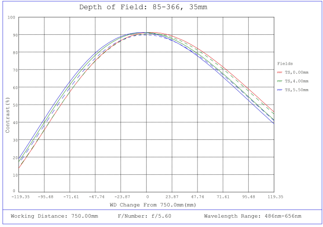
#85-366, 35mm, f/5.6 Ci Series Fixed Focal Length Lens, Depth of Field Plot, 750mm Working Distance, f5.6
