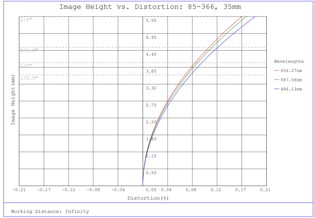
#85-366, 35mm, f/5.6 Ci Series Fixed Focal Length Lens, Distortion Plot
