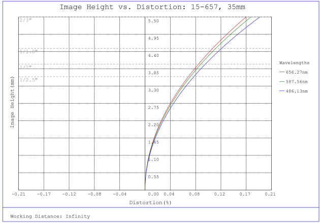
#15-657, 35mm, f/4 Cw Series Fixed Focal Length Lens, Distortion Plot
