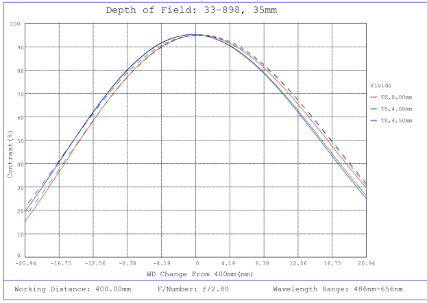
#33-898, 35mm f/2.8, UCI Series Fixed Focal Length Lens, Depth of Field Plot, 400mm Working Distance, f2.8
