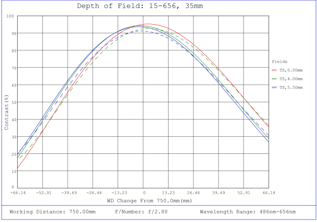
#15-656, 35mm, f/2.8 Cw Series Fixed Focal Length Lens, Depth of Field Plot, 750mm Working Distance, f2.8
