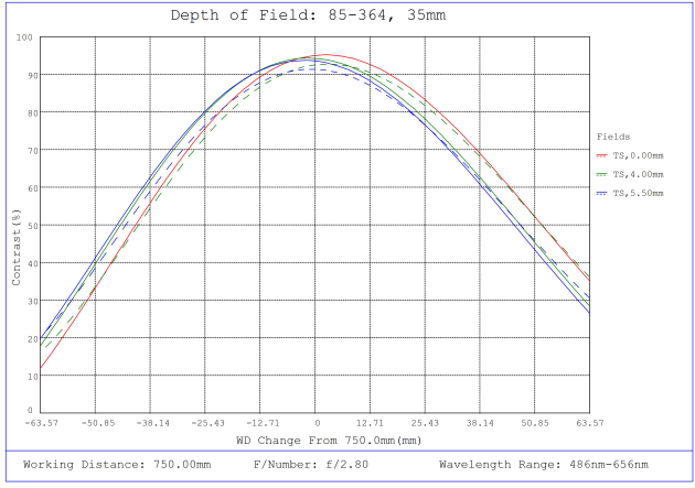
#85-364, 35mm, f/2.8 Ci Series Fixed Focal Length Lens, Depth of Field Plot, 750mm Working Distance, f2.8
