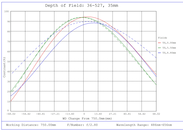
#36-527, 35mm f/2.8, HPr Series Fixed Focal Length Lens, Depth of Field Plot, 750mm Working Distance, f2.8
