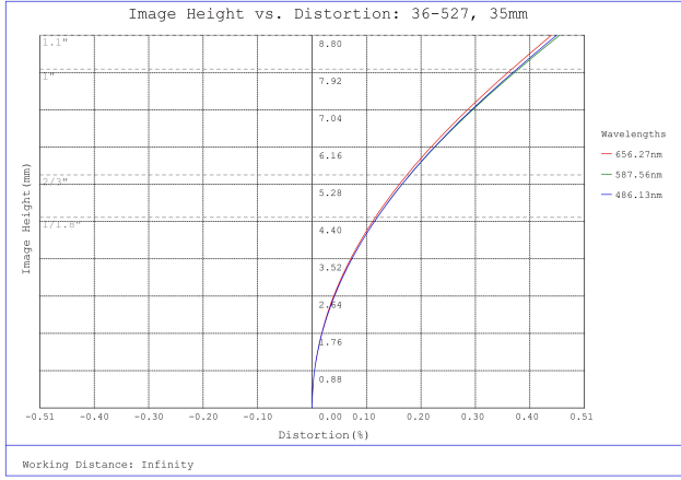
#36-527, 35mm f/2.8, HPr Series Fixed Focal Length Lens, Distortion Plot
