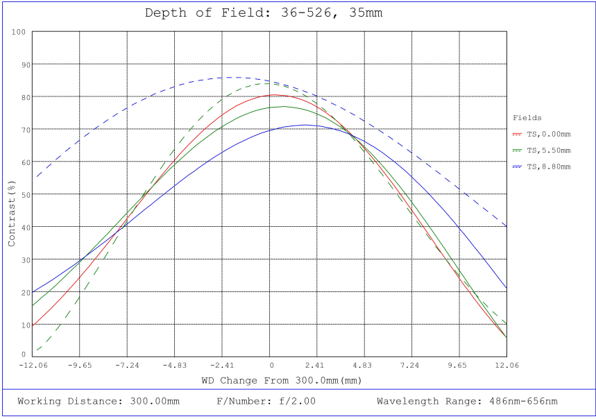
#36-526, 35mm f/2.0, HPr Series Fixed Focal Length Lens, Depth of Field Plot, 300mm Working Distance, f2
