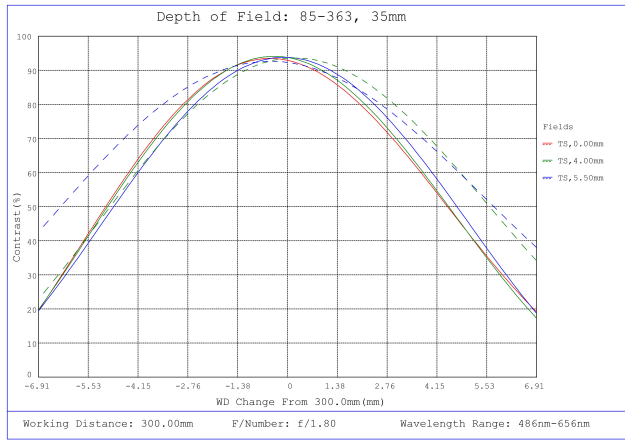
#85-363, 35mm, f/1.8 Ci Series Fixed Focal Length Lens, Depth of Field Plot, 300mm Working Distance, f1.8
