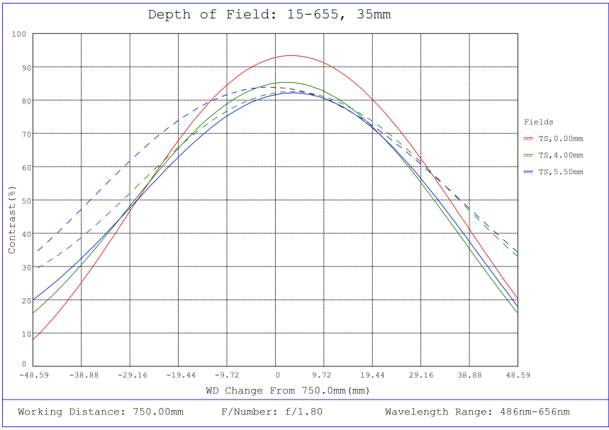
#15-655, 35mm, f/1.8 Cw Series Fixed Focal Length Lens, Depth of Field Plot, 750mm Working Distance, f1.8
