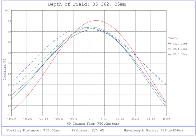
#85-362, 35mm, f/1.65 Ci Series Fixed Focal Length Lens, Depth of Field Plot, 750mm Working Distance, f1.6
