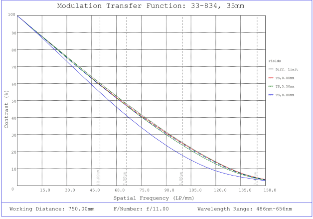
#33-834, 35mm f/11.0, HPI Series Fixed Focal Length Lens, Modulated Transfer Function (MTF) Plot, 750mm Working Distance, f11
