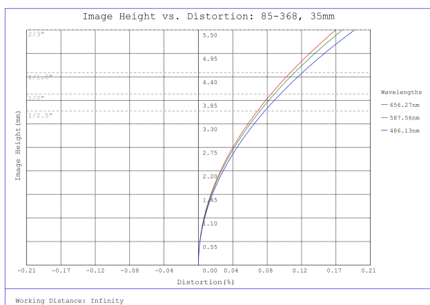
#85-368, 35mm, f/11 Ci Series Fixed Focal Length Lens, Distortion Plot
