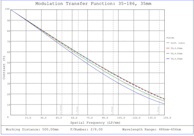
#35-186, 35mm, f/8.0 Cr Series Fixed Focal Length Lens, Modulated Transfer Function (MTF) Plot, 500mm Working Distance, f8
