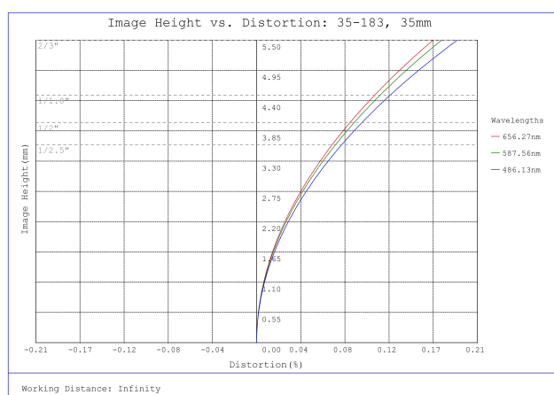
#35-183, 35mm, f/2.8 Cr Series Fixed Focal Length Lens, Distortion Plot
