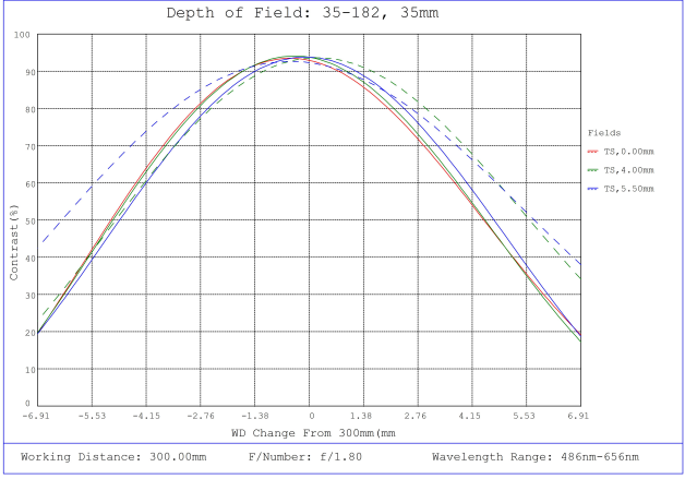
#35-182, 35mm, f/1.8 Cr Series Fixed Focal Length Lens, Depth of Field Plot, 300mm Working Distance, f1.8
