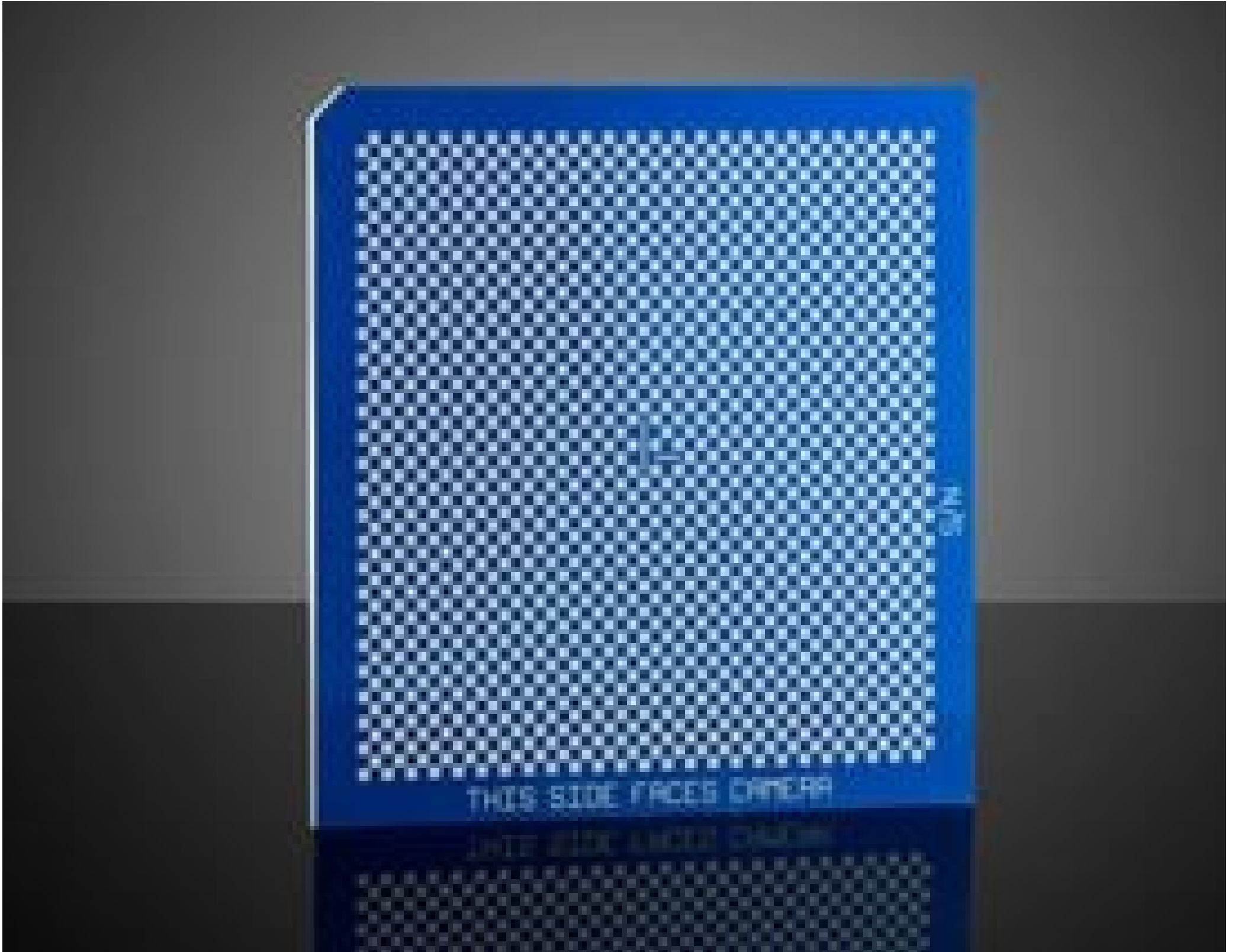
Opal Checkerboard Calibration Target
