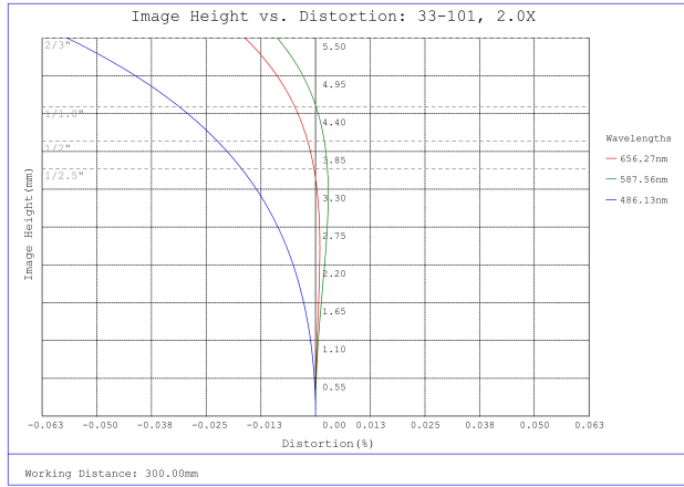
#33-101, 2X, 300mm WD CompactTL™ Telecentric Lens, Distortion Plot
