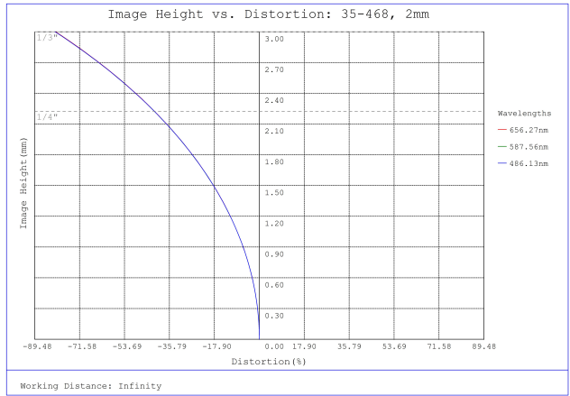
#35-468, 2mm FL f/8 IR-Cut, Blue Series M12 Lens, Distortion Plot
