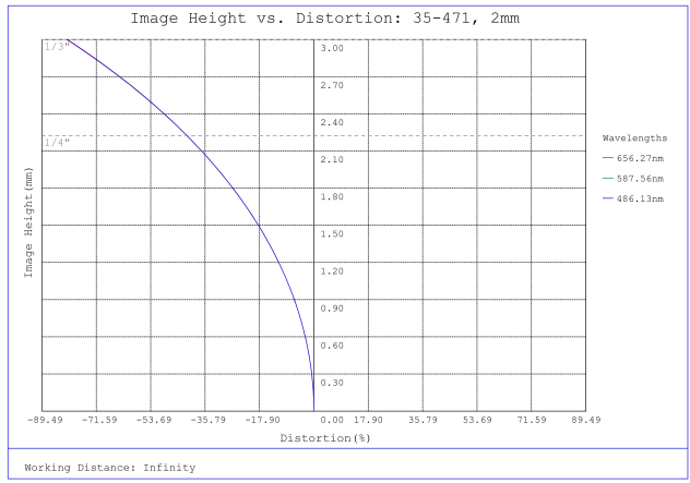
#35-471, 2mm FL f/5.6 IR-Cut Rugged Blue Series M12 Lens, Distortion Plot
