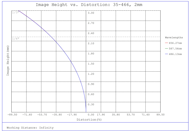
#35-466, 2mm FL f/4 IR-Cut, Blue Series M12 Lens, Distortion Plot
