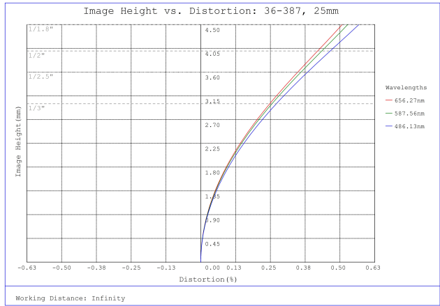
#36-387, 25mm FL f/8, Rugged Blue Series M12 Lens, Distortion Plot
